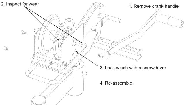
If wear is noticed, or re-tourquing does not resolve the issue, replace the winch assembly. NOTE: Die Lifter head shown, Mobile Crane winch is similar.
