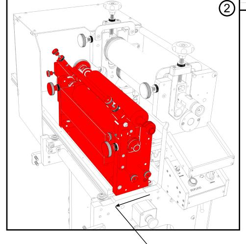
Move the print head assembly away from the machine and slide out to access rollers.
