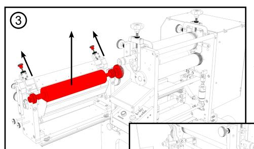
Unscrew the mount screws for the doctor blade assembly. Remove the doctor blade and lift out the meter roll.
