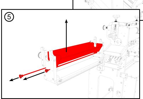
Remove the dowel pins affixing the ink tray. Lift our tray to remove.
