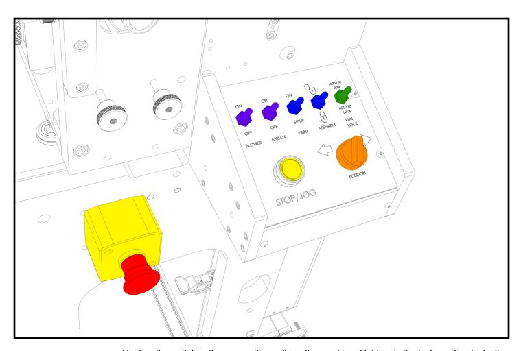
**RUN SWITCH**Holding the switch in the run position will run the machine. Holding in the lock position locks the press for roll maintenance.
