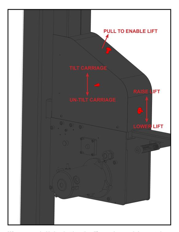
When equpped with the electric option, lift controls are switch operated.
