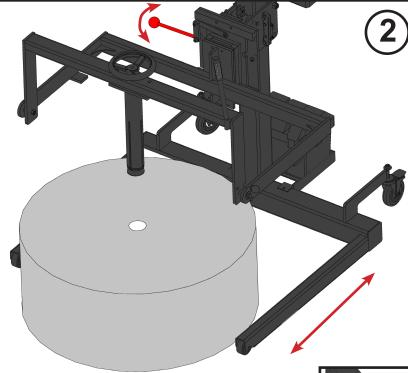
**2:** Move the cart into position over the roll. Use the side-lay handle to aid in positioning the roll.
