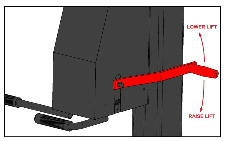
To operate the lift, turn crank handle clockwise to raise and counter-clockwise to lower. When raising the lift, make certain that the winch makes a clicking sound.
