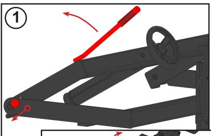
**1:** Pull the pin retaining the core holder. Rotate to vertical position. Release pin to lock.
