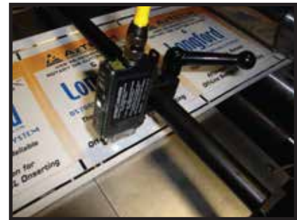
Electronic Web Sensor for Precise Registration and placement
