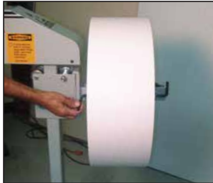
Manually activated roll stop to prevent roll from falling off attachment
