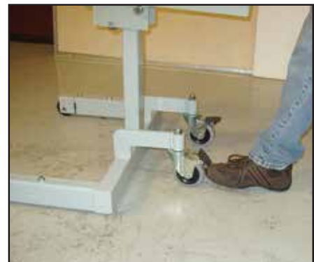
Toe activated wheel safety brake to secure cart in desired position
