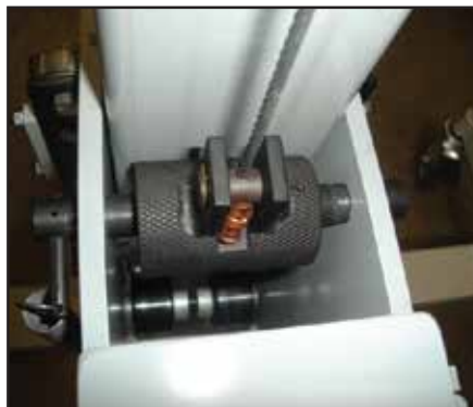
Automatically activated safety brake to prevent load drop in event of cable breakage
