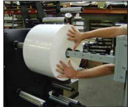
Easily load and remove rolls utilizing roller core attachment
