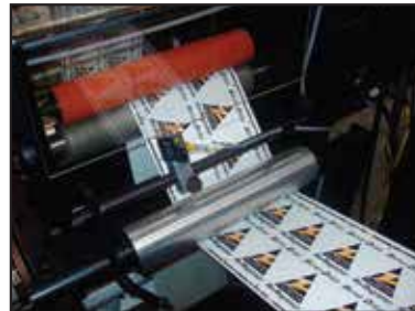
Adjustable sensor electronically sends web corrections to the servo-drives.
