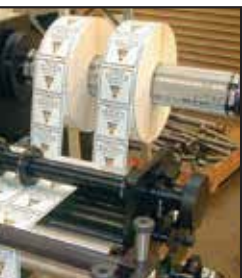
Finished roll dual-rewind spindles and slitting station shown with rotary shear knives. Also available with pneumatic rotary crush knives, and razor slitting.
